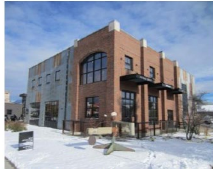
Figure 20.131.060.C.2 Acceptable metal siding examples.
