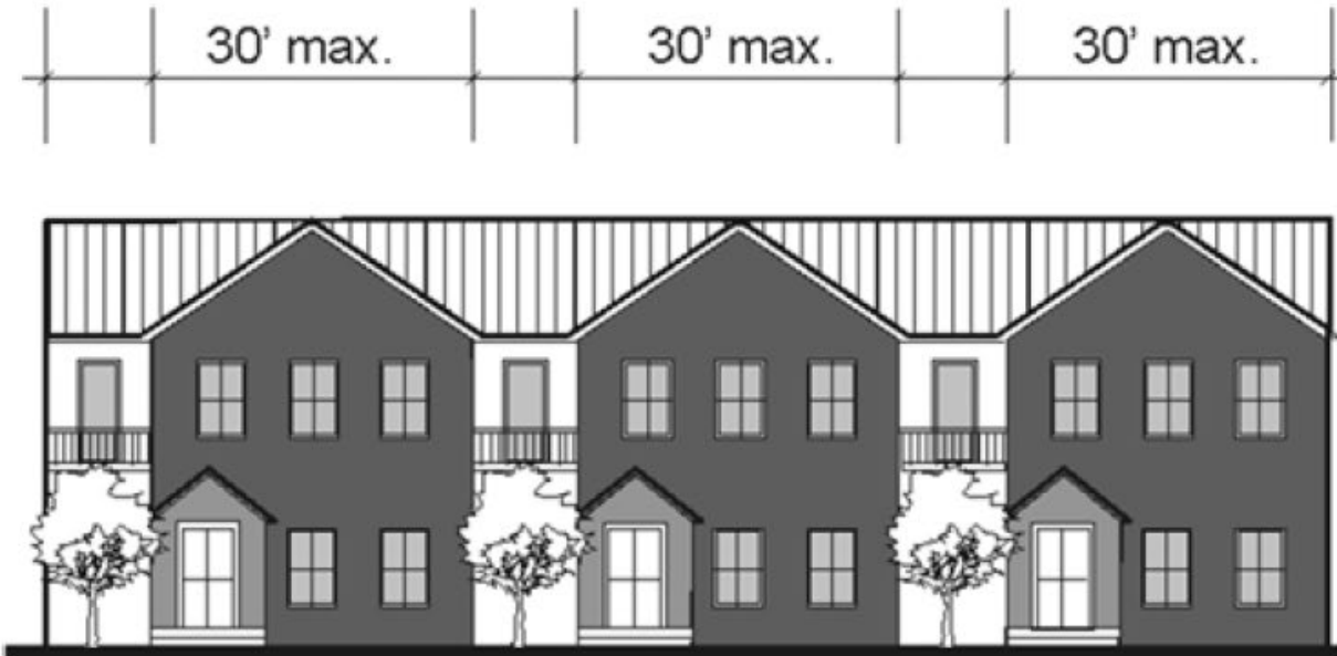
Figure 20.131.040.C Residential façade articulation examples.
